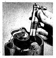
4. Replace cartridge-pistol and screw tight, making sure safety pin is pushed in.
