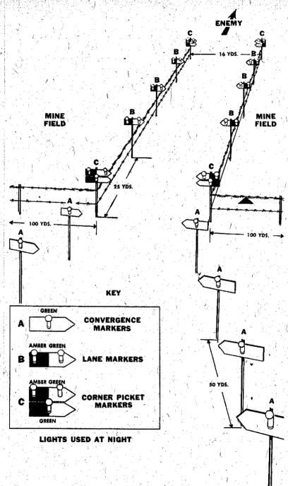
Figure 43.09a. Mine-field lane marking.
