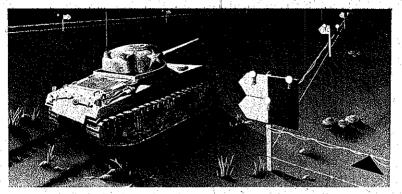
Figure 43.09b. Night view of mine-field lane marking.
