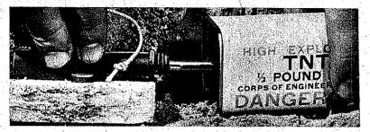
7. Remove safety clip. It should pull off easily. A sudden jerk may cause fuze to fire. If safety clip does not pull off easily, check installation to make sure there is no pressure on pressure cap.
