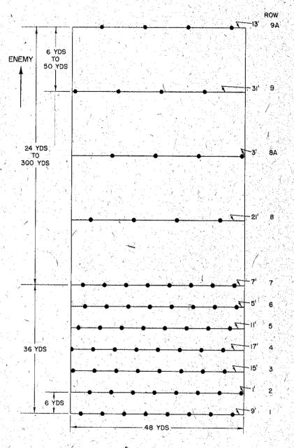
Figure 32.02d. Extended section, deliberate mine belt.
