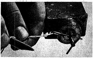
2. If mine is set for firing by trip wire, cut wire.
