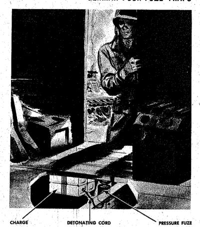
Germans leave booby traps for the unwary to tread on, particularly in populated places but also in the fields. The fuze may be either D. Z. 35, S. Mi. Z. 35, or Es. Mi. Z. 40. The charge may be an "S" mine, a grenade, one or more slabs of tolite, a Tellermine, or a shell or bomb. To find and disarm these traps.
