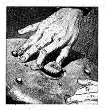
2. Turn safety screw tight, clockwise, until line marked SICHER coincides with white mark on case.
