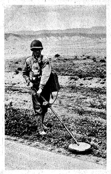
Figure 1.2. Electrical mine detector.
