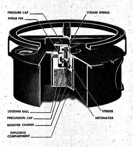
The antitank mine M1, the original model, is no longer being manufactured or issued. It is handled exactly the same as the antitank mine M1A1.
