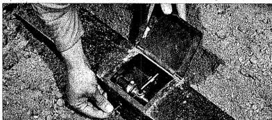
2. Insert strong wire through safety pin hole in side of cover, case, and fuze housing.
