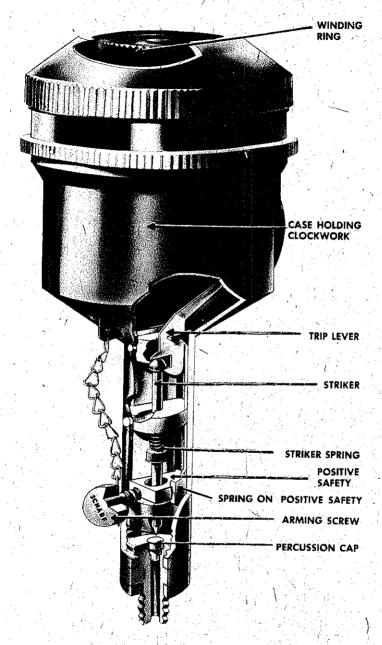
1. At end of delay period, lever arm on rotating control disk in clockworks bears against trip lever, disengaging striker.
