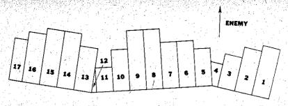
Figure 32.02e. Mine belt laid with extended pattern sections.
