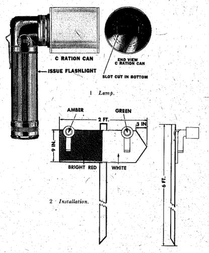
Figure 43.09c. Improvised mine-field lane-marker lamp.
