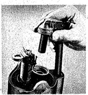
6. Insert detonator, small end first, so cap end rests on shoulder in socket.
