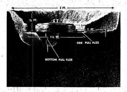
The Germans usually booby-trap mines to make removal of their mine fields and road blocks more hazardous and time-consuming. The number booby-trapped depends upon the time spent in laying the field, and on its importance. For this purpose the Tellermines have two secondary fuze wells, one in the side and the other in the bottom. (See sections 81.01–81.04, Tellermines.) Any of the standard pull fuzes, with detonator attached, fits into these wells.
