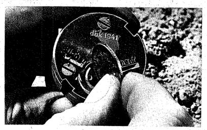
1. After disarming, remove fuze and turn dial from SCHARF to SICHER. Use coin or knife—not screwdriver.
