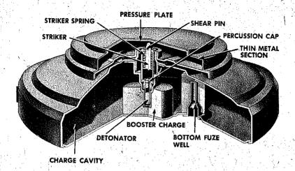
T. Mi. 43 (mushroom) is a modification of T. Mi. 42 (page 81.03), uses same fuze (T. Mi. Z. 42), and is handled same way. Principal difference is that the entire pressure plate T. Mi. 43 (mushroom), rather than just hexagonal cap as in T. Mi. 42, unscrews to uncover fuze. Initial resistance to pressure is provided by thin walls of pressure plate rather than by an inner spring.
