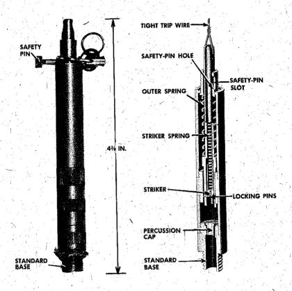
TYPE. Either pull or tension-release fuze
