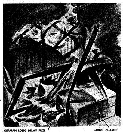
A favorite German trick is to leave large charges of explosive -as much as 2,000 pounds-in abandoned buildings. Basements are favorite locations, though stoves, furnaces, chimneys, attics, and cupboards have been used. Clockwork fuzes are used, set for delays from several hours to many days. To find and disarm this type of booby trap-
