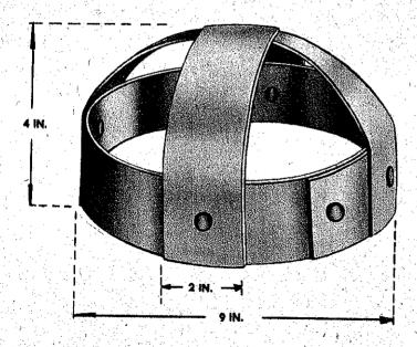
Figure 21.08d. Individual mine marker.
