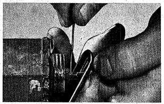
If mine is set with free safety hole on inside, hence not visible, grasp striker firmly and pull out until free hole is visible.
