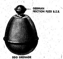
German grenades employ a friction fuze with a 4½-second delay pellet so the grenade reaches the target before exploding. Friendly troops using captured grenades sometimes find they explode immediately upon pulling the friction wire. This means grenades have been booby-trapped by removing the delay pellet. Before using captured grenades, examine as follows:
