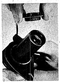
1. Unscrew safety cap from base of fuze and examine fuze to see that it is not broken or otherwise unserviceable.
