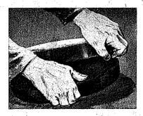
**3.** Remove tape from joint between covers, and pry loose bottom cover.
