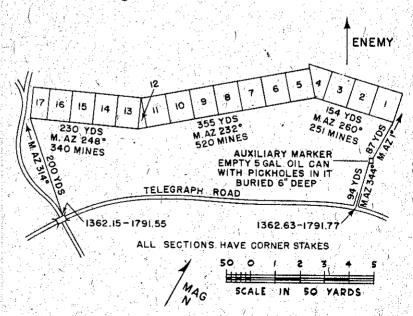
Figure 32.01. Lay-out of typical deliberate mine belt.
