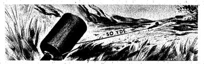
3. Pull mine and stake loose with 50-yard length of wire. Stake may be booby-trapped.
