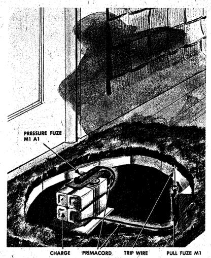
Sketch shows typical combination pull- and pressure-fuze installation.
