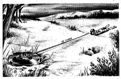
2. Pull out mine with 50 yards of rope or wire; or, search for and disarm secondary fuzes (page 85.01-a), and then lift mine.
