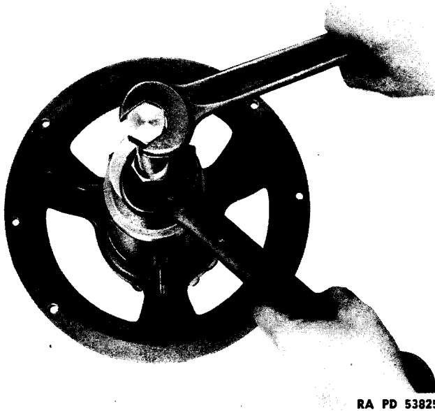
Figure 26 — Assembling Crankshaft, Using Fixture HL-AA-205 (2)
