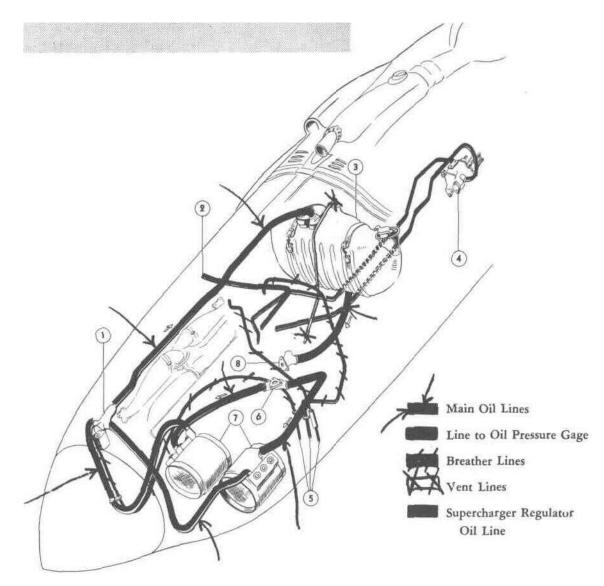
Figure 19 — Oil System Diagram
