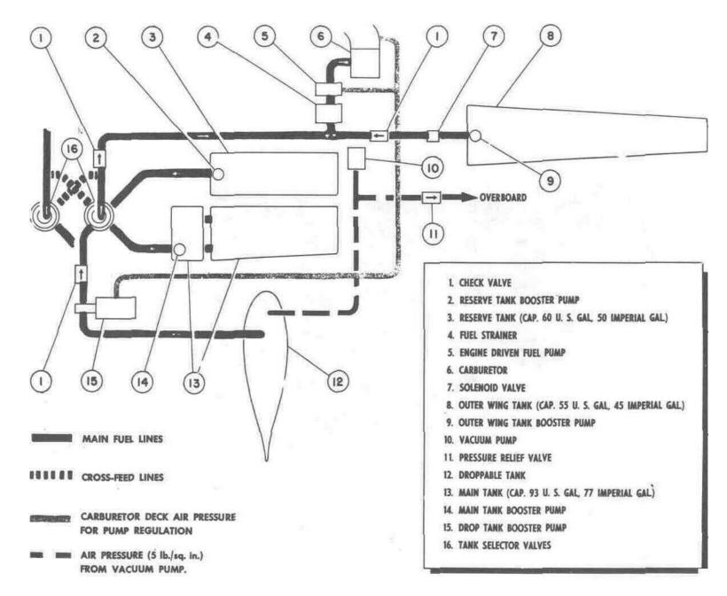
Figure 10A — Simplified Fuel System Diagram (Modified Airplanes)
