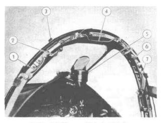
1. Hatch locking arm (locked position).
