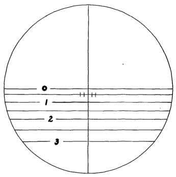
FIGURE 16 .--- Telescope reticle.
