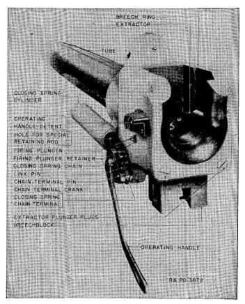
FIGURE 3.—75-mm tank gun M2—rear, breech in full open position.
