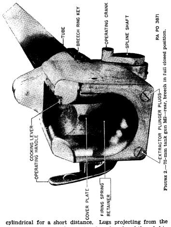
cylindrical for a short distance. Lugs projecting from the top and bottom near the front end are bored and threaded to receive the piston rods of the recoil and counterrecoil mechanism. The bottom lug extends rearward on either side of the bottom of the breech ring and is bored transversely to provide bearings for the operating and chain terminal cranks.
