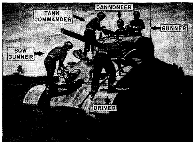
Figure 2. Mounting through hatches, medium tank with single turret hatch.
