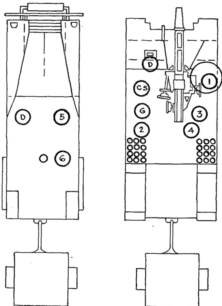
FIGURE 7.—Posts of section, mounted, 105-mm motor carriage M-7.
