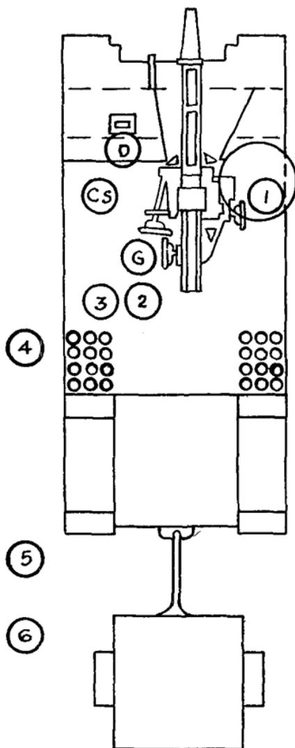
FIGURE 9.—Post of cannoneers prepared for action, 105-mm howitzer motor carriage M-7. (The ammunition carrier is placed for perimeter defense and the driver mans the caliber .30 machine gun.)
