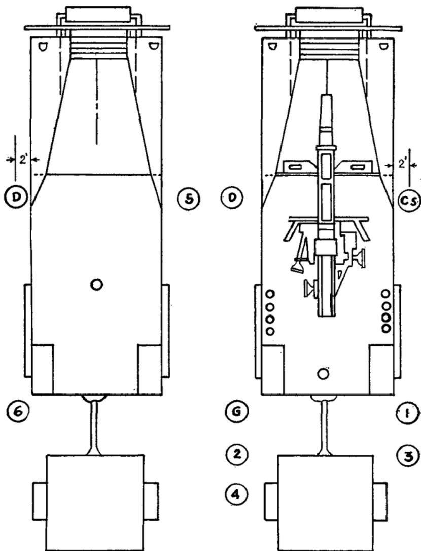
FIGURE 4.—Posts of section, dismounted, 105-mm howitzer motor carriage T-19.
